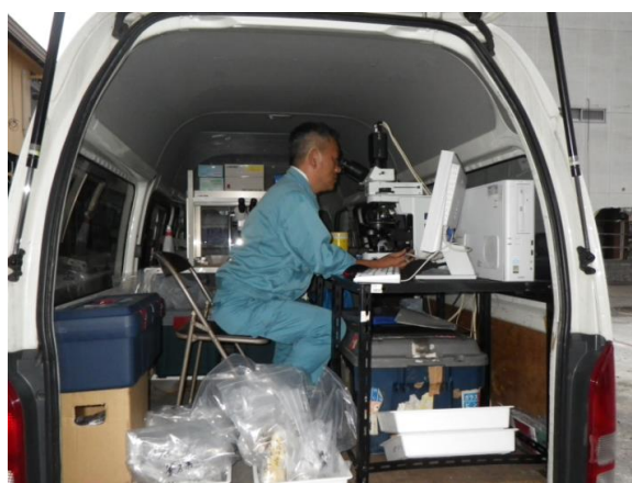
Figure 3 Asbestos analysis on site
