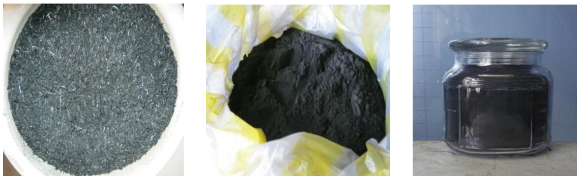
Figure 1. (from left to right) Original sample, Sample after grinding and sifting, Preservation of samples
