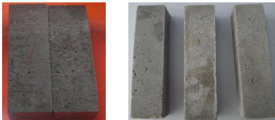
Figure 6. Raw Sample and Refined sample after soaking with water 28 days
