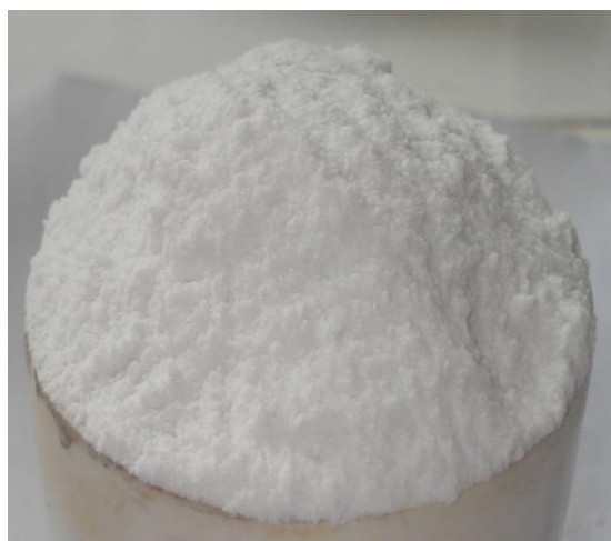
Figure 5. SiO 2 extracted from rice husk ash
